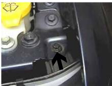
**2.** Using the 7MM socket, remove two metric bolts from the top of head light assembly, pull forward, both sides, and set a side.
